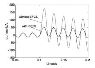
Fig.4: The fault current characteristics waveform (mode 1).
