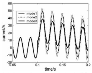
Fig. 5: The fault current characteristics comparison in all three modes.
