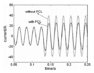
Fig. 10: Fault current characteristics waveforms.
