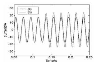
Fig.11: The characteristics of current for the seconding winding according to:(a) normal state and (b) fault state.
