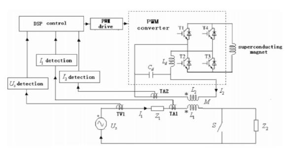
Fig.1: circuit arrangement of the active SFCL
