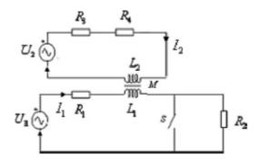
Fig.9: Experimental circuit of the FCL.  $L_1 = 5.98$  mH;  $L_2 = 5.92$  mH; M = 5.87 mH;  $R_1 = R_3 = 0.6$   $\Omega$ ;  $R_2 = R_4 = 0.8$   $\Omega$ ;  $|\dot{\textbf{U}_1}| = |\dot{\textbf{U}_2}| = 25$  V.
