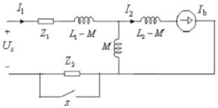
Fig.3: Active SFCL equivalent circuit
